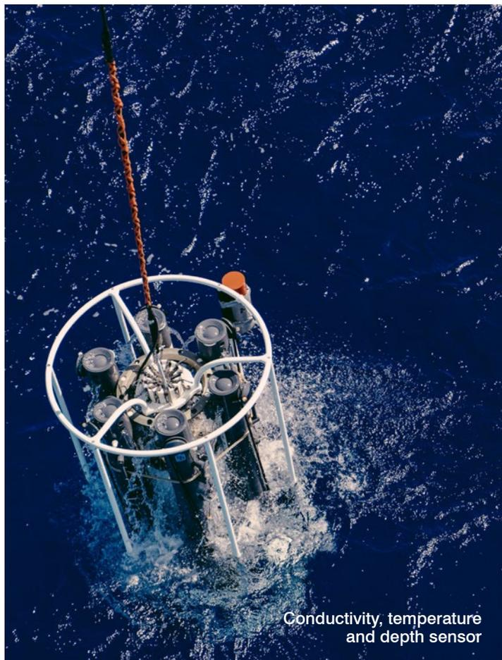
Conductivity, temperature and depth sensor
