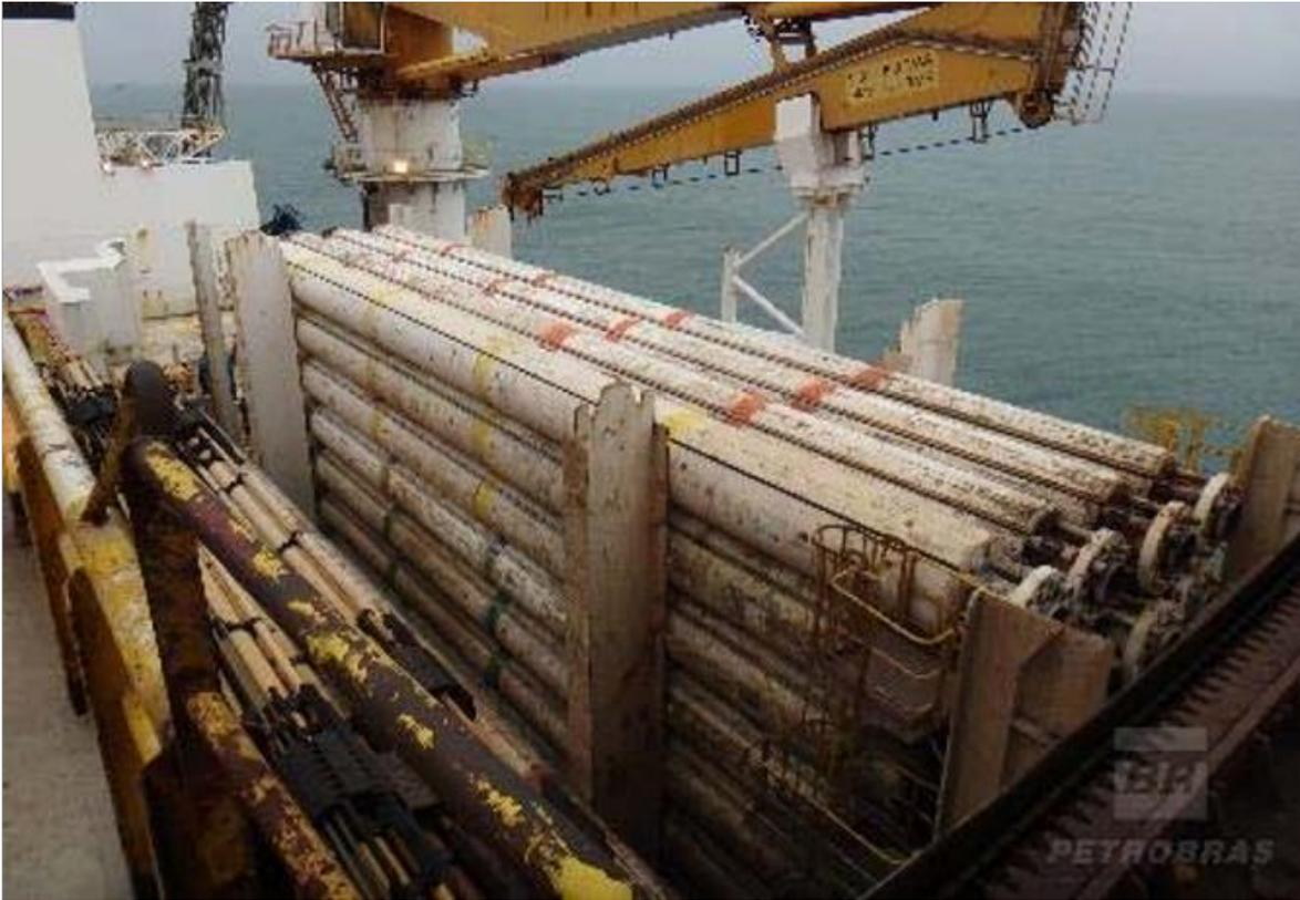
A riser joint is loaded on to trolley cradle and skate moved towards the moon pool. The riser is upended by hanging it from the riser running tool that is suspended from the top drive. The riser is lowered/pulled up with a winch. When the desired position is reached, the arms of the lifting tool are lowered to support the riser. The riser running tool is disconnected to pick up the next riser joint to be installed.
