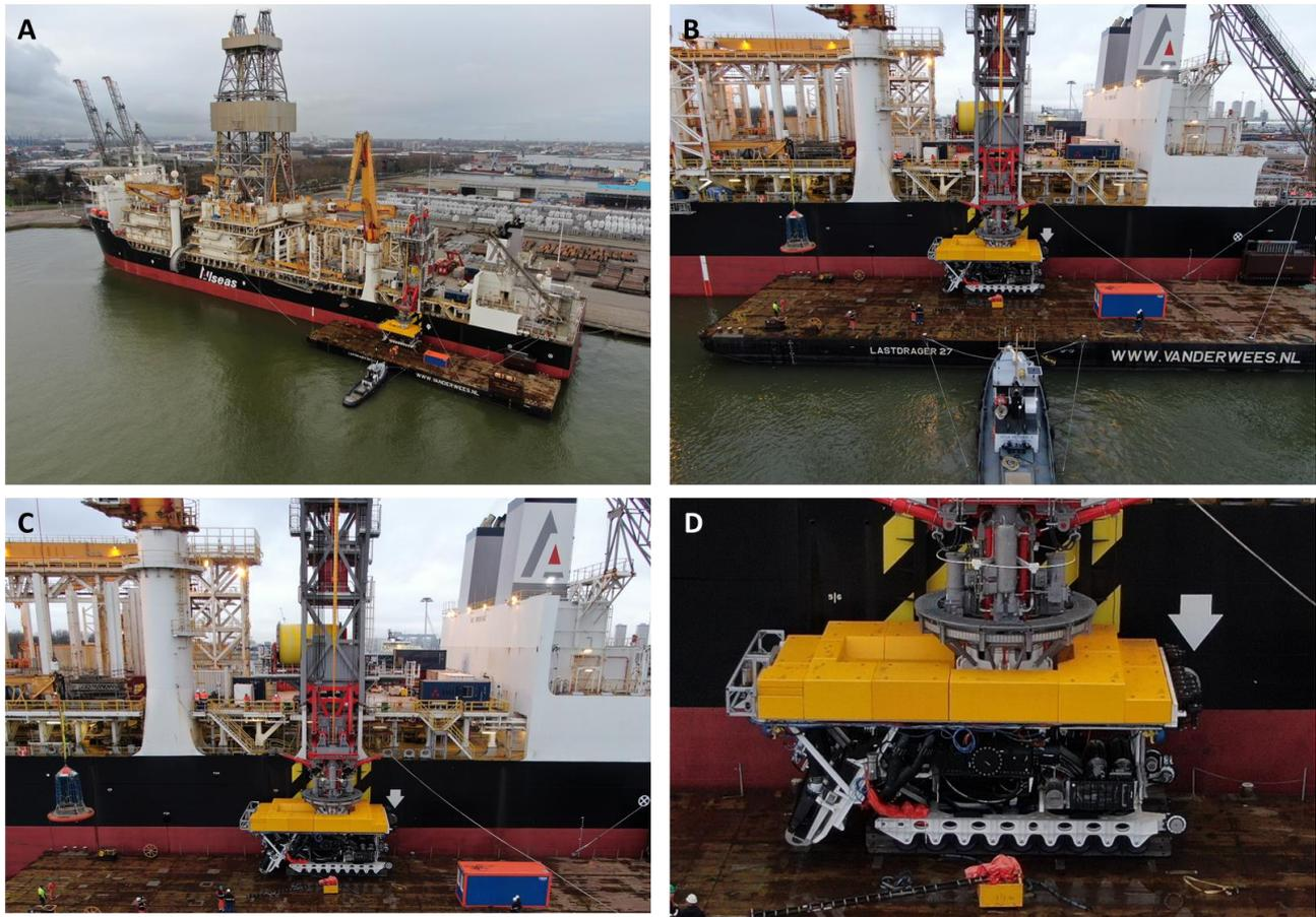
**Note:** A - Hidden Gem; B - LARS system; C - LARS system and Prototype Collector Vehicle; D – Prototype Collector Vehicle
