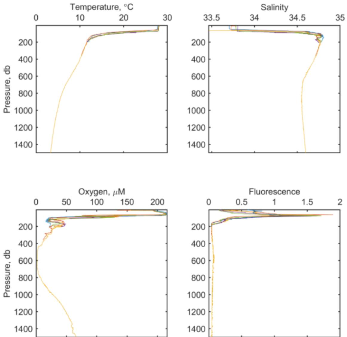
Figure 5-40. Vertical profiles of temperature, salinity, dissolved oxygen, and fluorescence in the upper 200 m of the water column at the CTA site during Campaign 5B.
