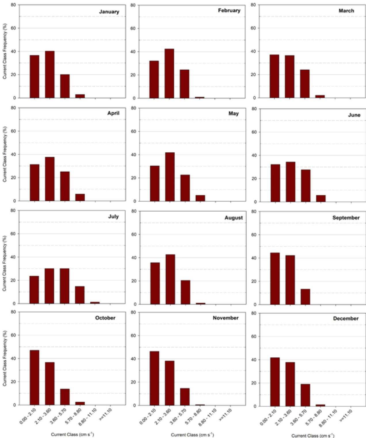
Figure 5-23. Near-continuous record of current speeds (cm s<sup>-1</sup>) and direction (flowing towards) recorded from bin #4 of upward-looking acoustic Doppler current profiler (ADCP) (300 kHz) at 2,000 m on the Long Mooring between 15 October 2019 and 2 June 2021.
