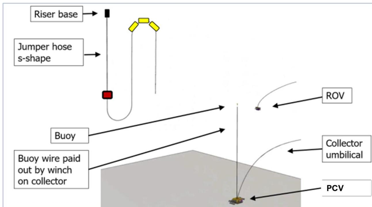
3. The jumper hose is pulled down to the PCV. The ROV guides the jumper connector on the hose in the horizontal plane, while the wire pulls in the hose.
