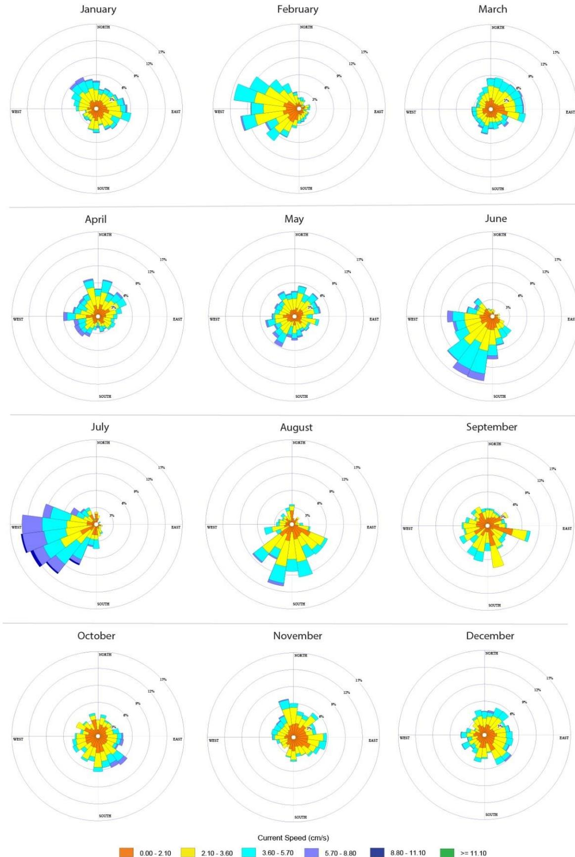
(b) Current speed and direction near seafloor (4,321 m water depth/5 m above seafloor)
