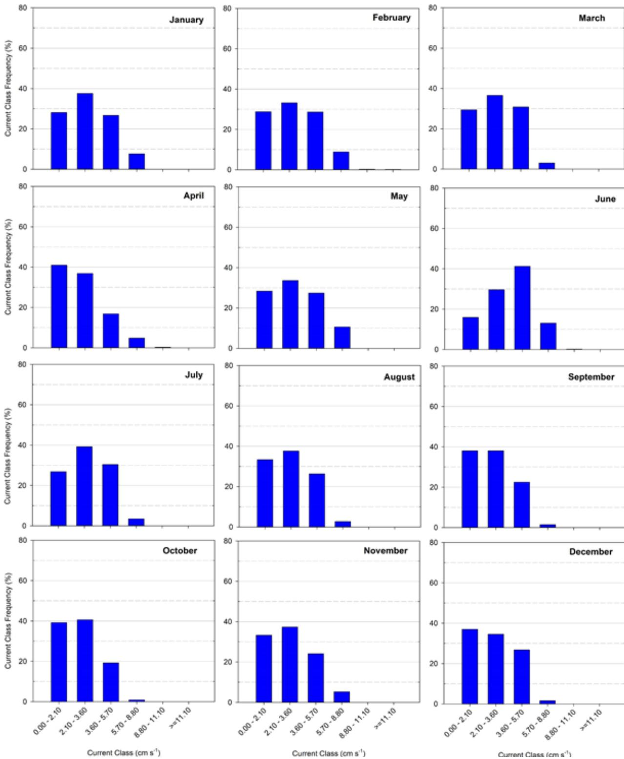
Figure 5-27. Near-continuous record of current speeds (cm s<sup>-1</sup>) and direction (flowing towards) recorded from bin #4 of the downward looking Acoustic Doppler Current Profiler (ADCP) (600 kHz) at 4,321 m water depth (i.e., 5 m above the seafloor) on the Long Mooring.
