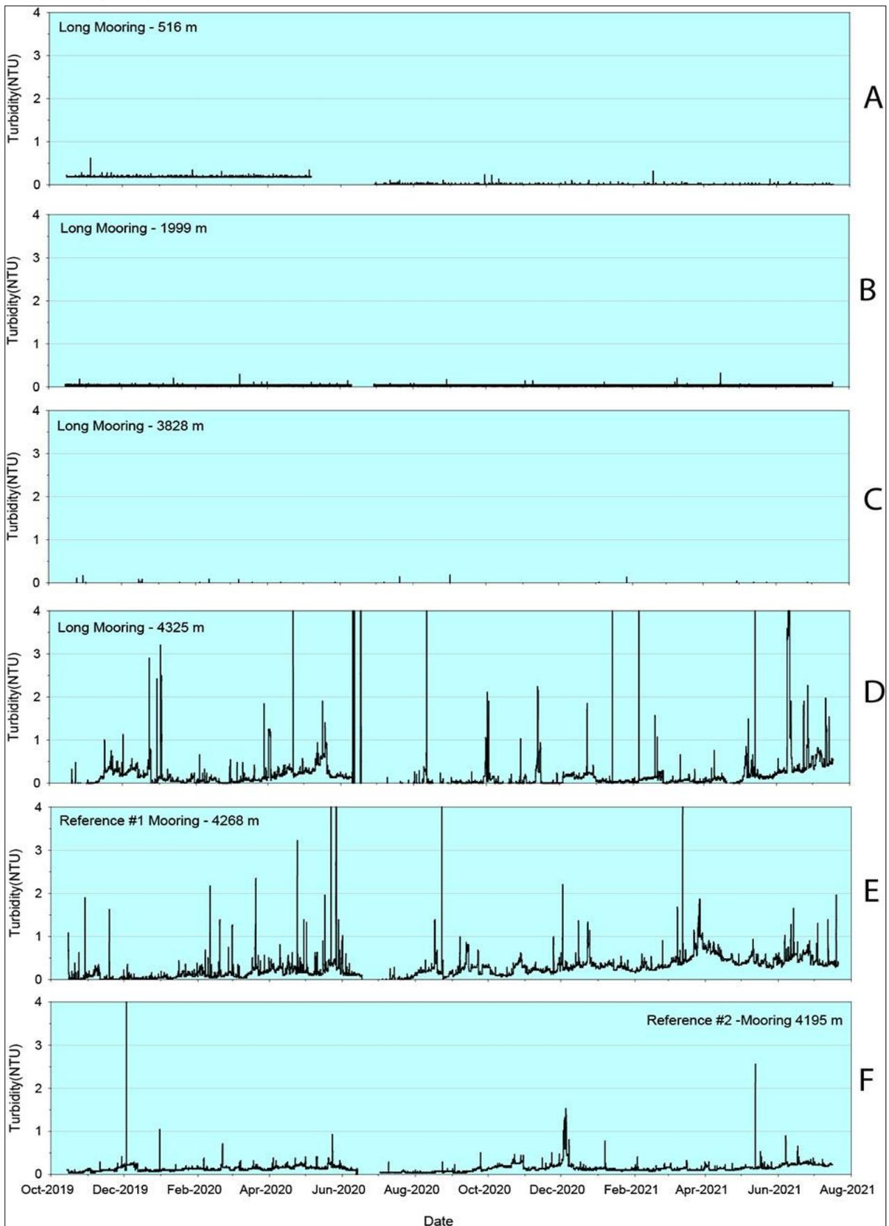
Figure 5-19. Near-continuous turbidity values (NTU) near-seafloor (i.e., <3.5 m above seafloor) with y axis showing the maximum values at the Long (red) and Reference (orange and brown) mooring stations from October 2019 through July 2021.
