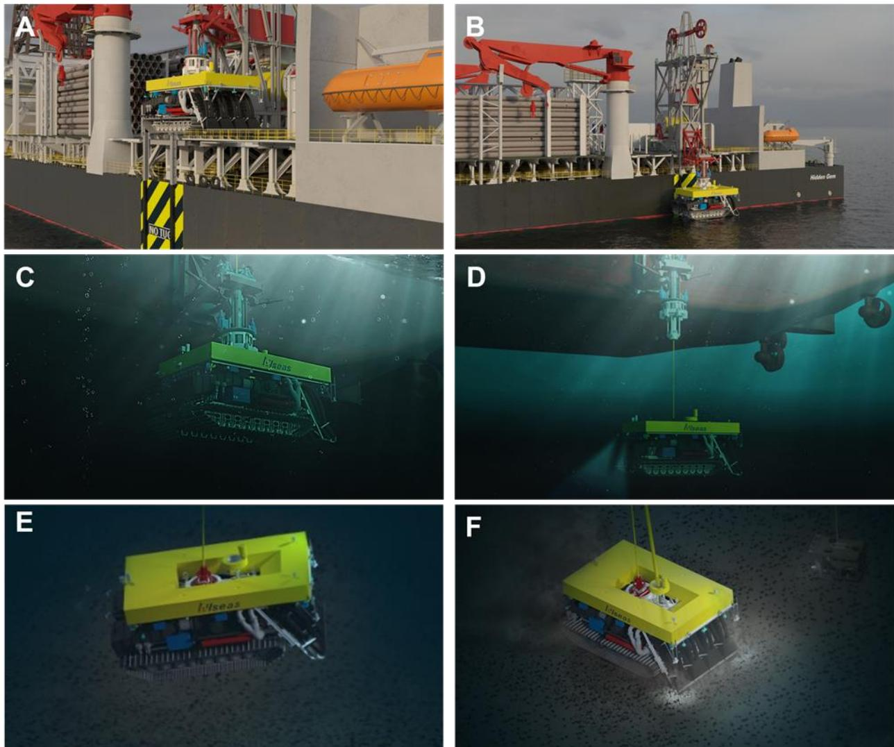
When lowering the PCV through the splash zone, the vessel heading will be adjusted such that the LARS is on the lee side, and wave shielding is provided to the LARS. This is done to reduce the splash zone loads, as illustrated in Figure 3-23. When the PCV has passed through the splash zone, the heading will be adjusted to bow incoming waves again.
