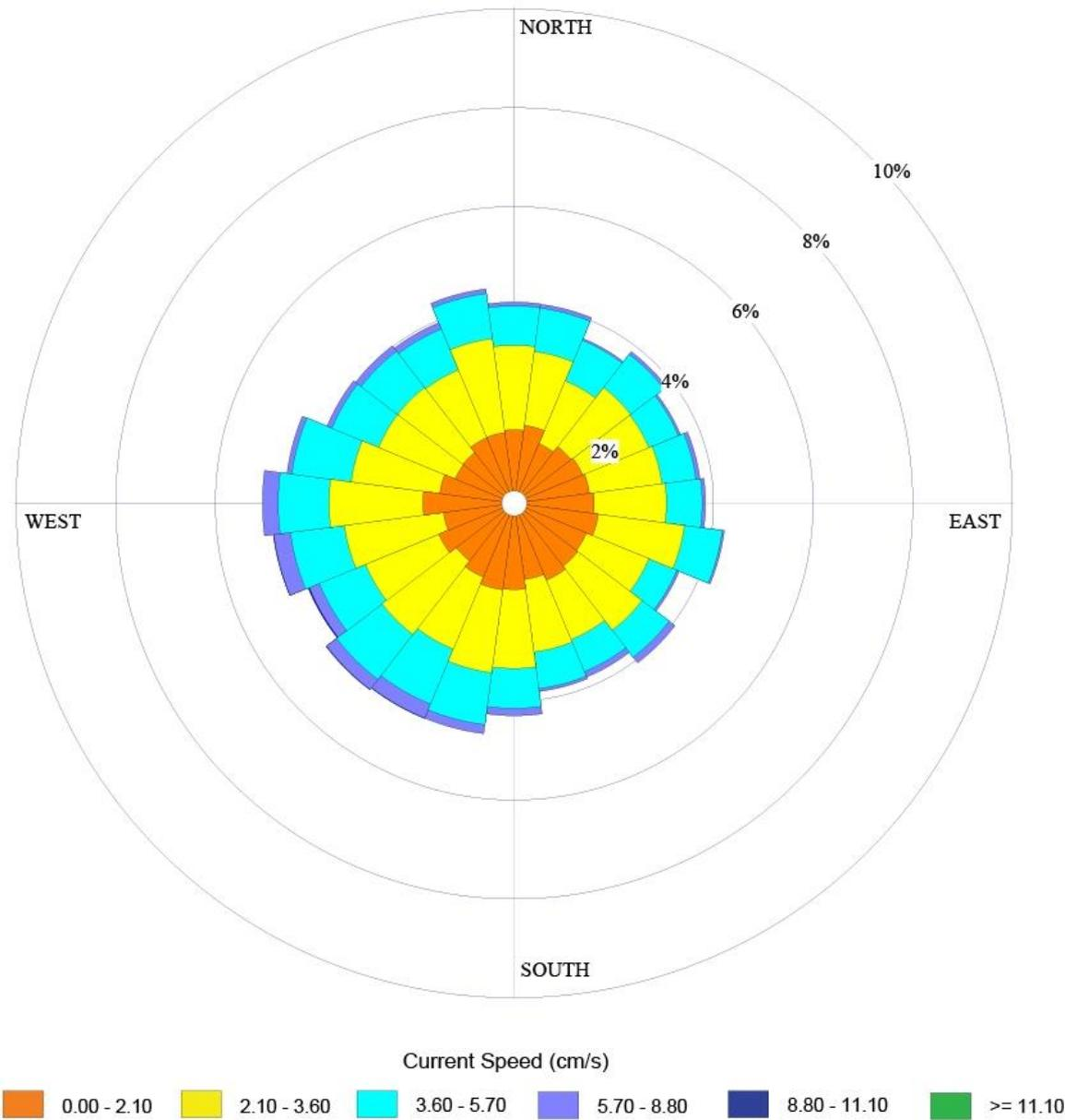
Figure 5-24. Monthly current rose direction (flowing towards) and speed (cm s<sup>-1</sup>) plot recorded from bin #4 of upward-looking acoustic Doppler current profiler (ADCP) (300 kHz) at 2,000 m on the Long Mooring between 15 October 2019 and 2 June 2021.
