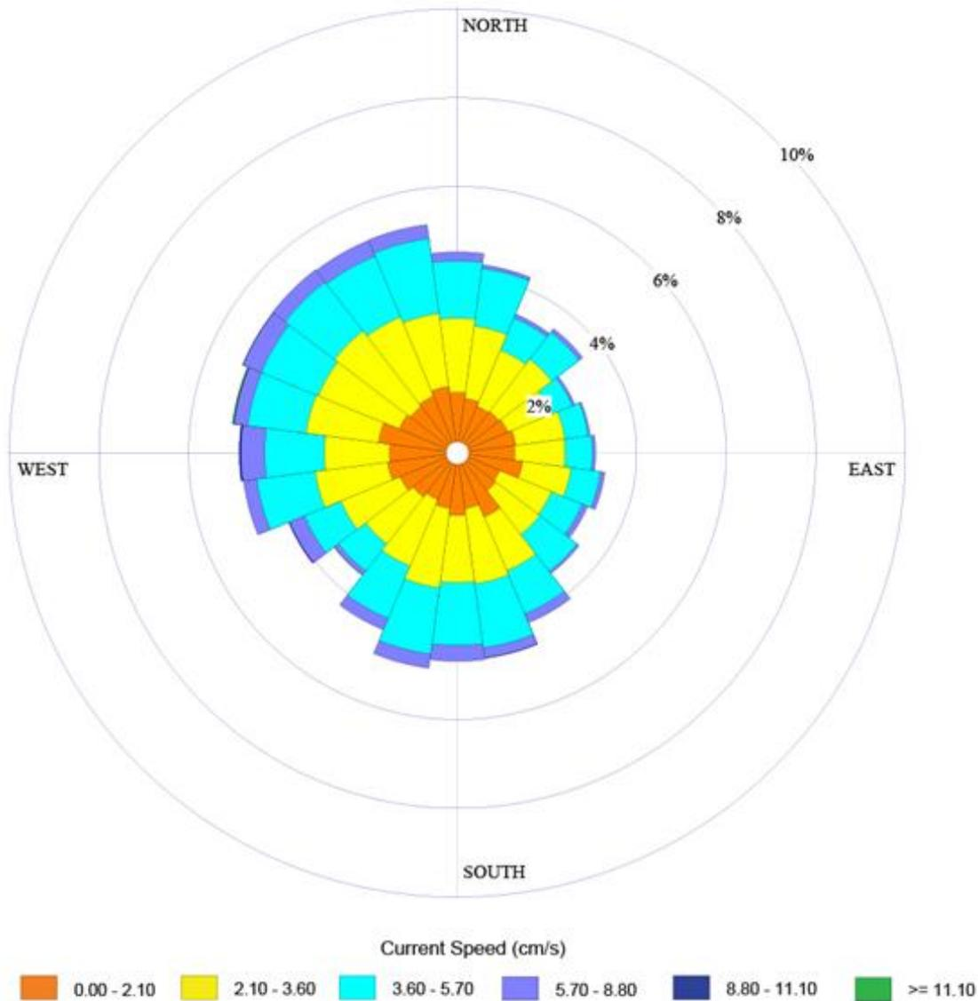
Figure 5-28. Monthly current rose direction (flowing towards) and speed (cm s<sup>-1</sup>) plot recorded from bin #4 of the downward-looking Acoustic Doppler Current Profiler (ADCP) (600 kHz) at 4,321 m water depth. (i.e., 5 m above the seafloor) on the Long Mooring between 15 October 2019 and 24 April 2021.
