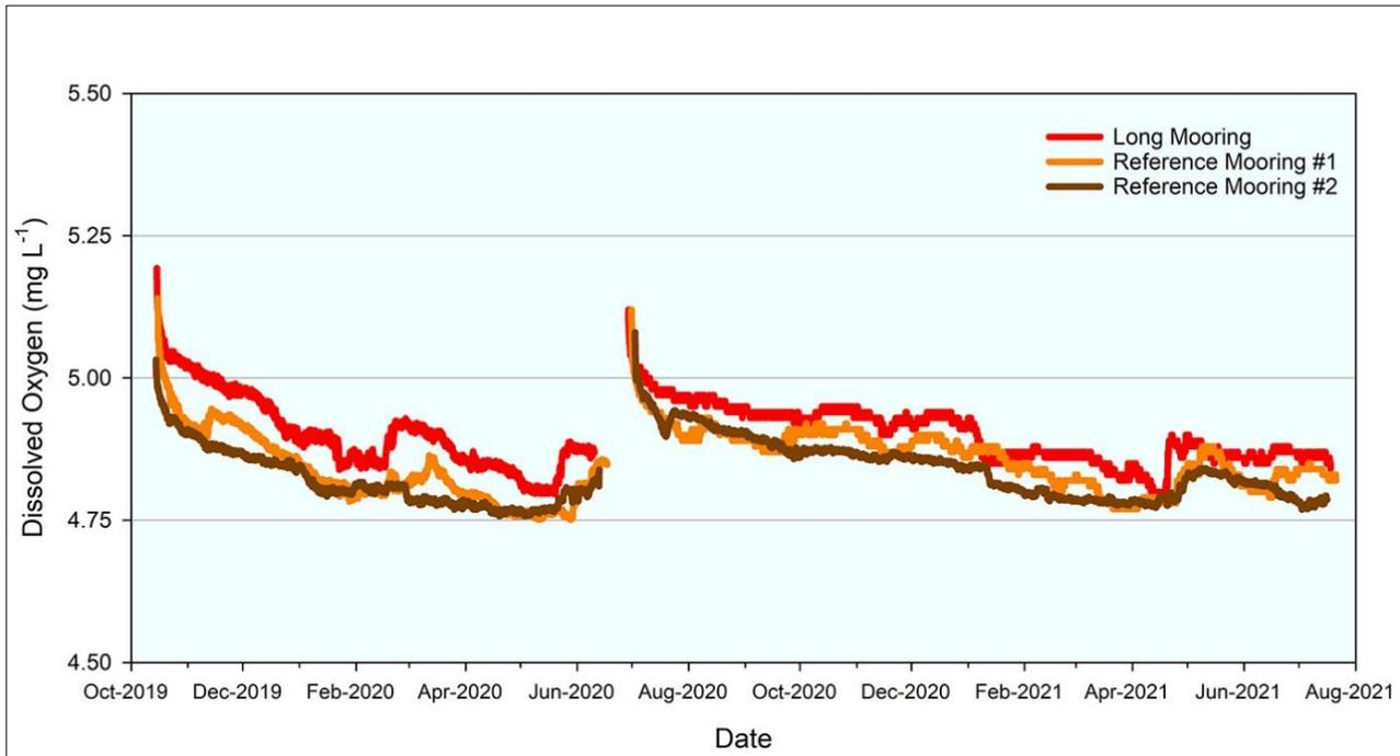
Figure 5-17. Running average of dissolved oxygen concentration values (mg L<sup>-1</sup>) by month at the proposed discharge water depth (~2,000 m) at the Long Mooring Site in the NORI-D block from October 2019 through July 2021.
