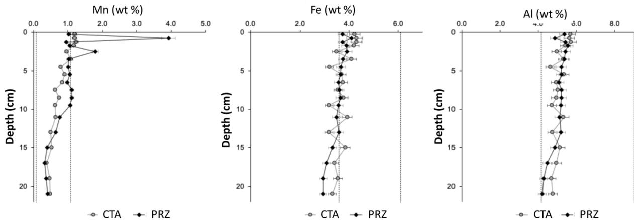
Note: Data still requires a minor correction for residual salt content. Dashed lines represent range observed in the CCZ in scientific literature (Volz *et al.*, 2018).
