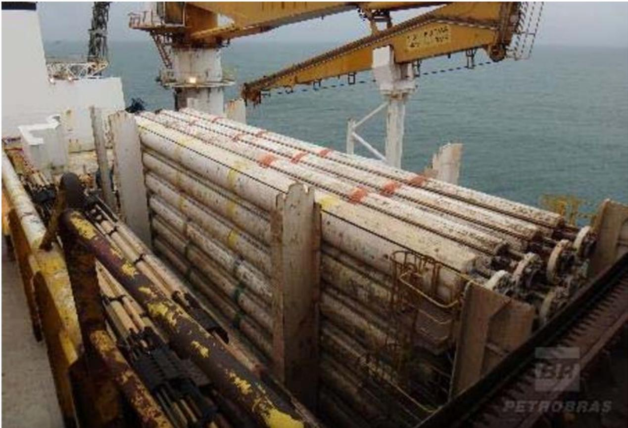
A riser joint is loaded on to trolley cradle and skate moved towards the moon pool. The riser is upended by hanging it from the riser running tool that is suspended from the top drive. The riser is lowered/pulled up with a winch. When the desired position is reached, the arms of the lifting tool are lowered to support the riser. The riser running tool is disconnected to pick up the next riser joint to be installed.
