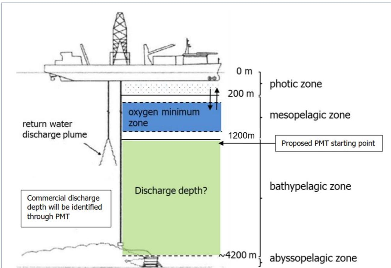
In the context of the Collector Test, placement of the return water discharge outlet at 1,200 m was based on the best information available at the time of design. The Collector Test will be used as an opportunity to accurately quantify depth of the neutrally buoyant plume and an adjustment to the discharge depth will be made for future operations, if required.
