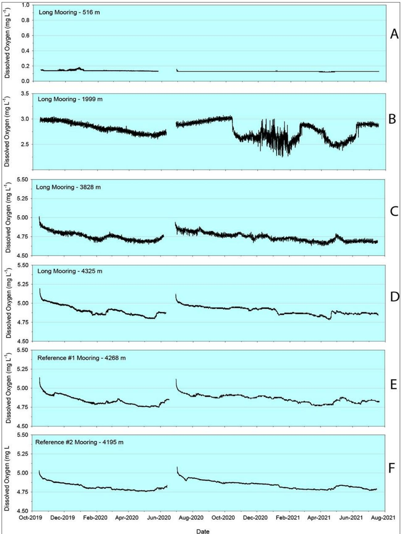
Figure 5-16. Near-continuous dissolved oxygen values (mg L<sup>-1</sup>) near-seafloor (i.e., <3.5 m above seafloor) at the Long (red) and Reference (orange and brown) mooring stations from October 2019 through July 2021.
