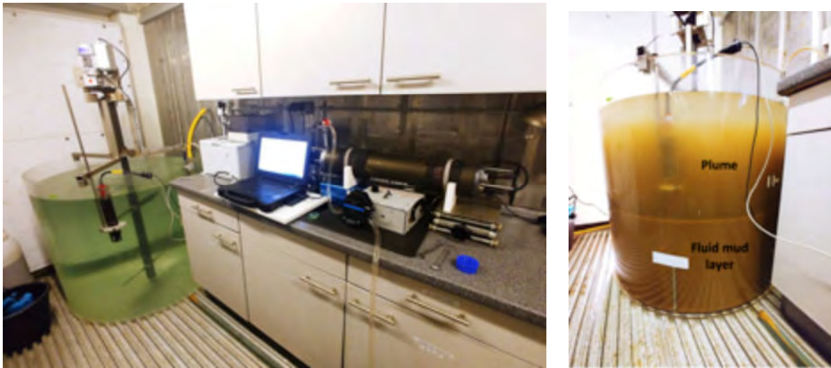
Fig. 2. Experimental setup in cool-room and water column simulator with developing mud layer
