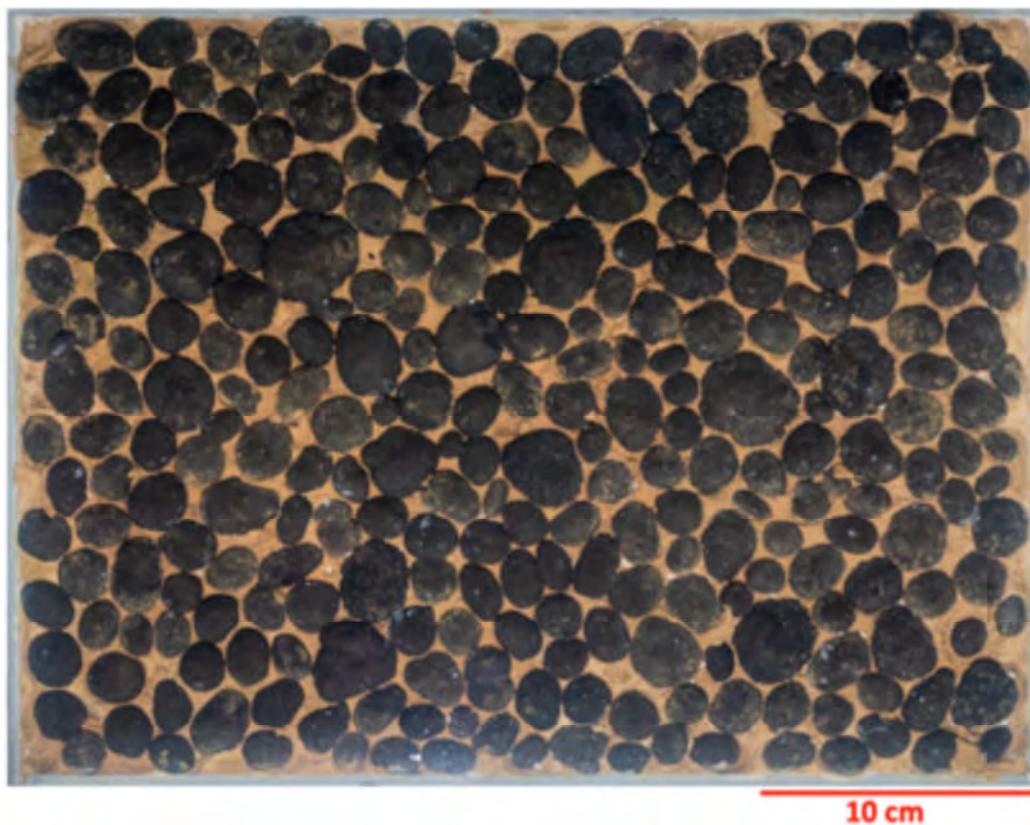
Fig.4. Test section, with 286 Type 1 nodules from the NORI exploration site ( \approx 16 kg ww)
