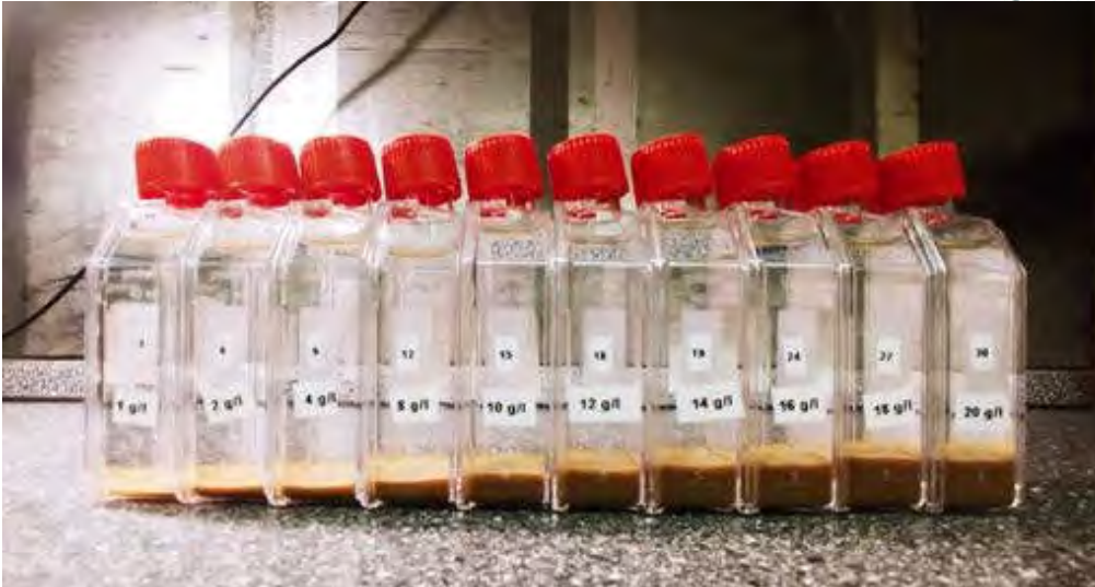
Fig. S3 Test vials for fig. 15. Aggregated plume particles were inserted to determine the height of the resulting mud layer
