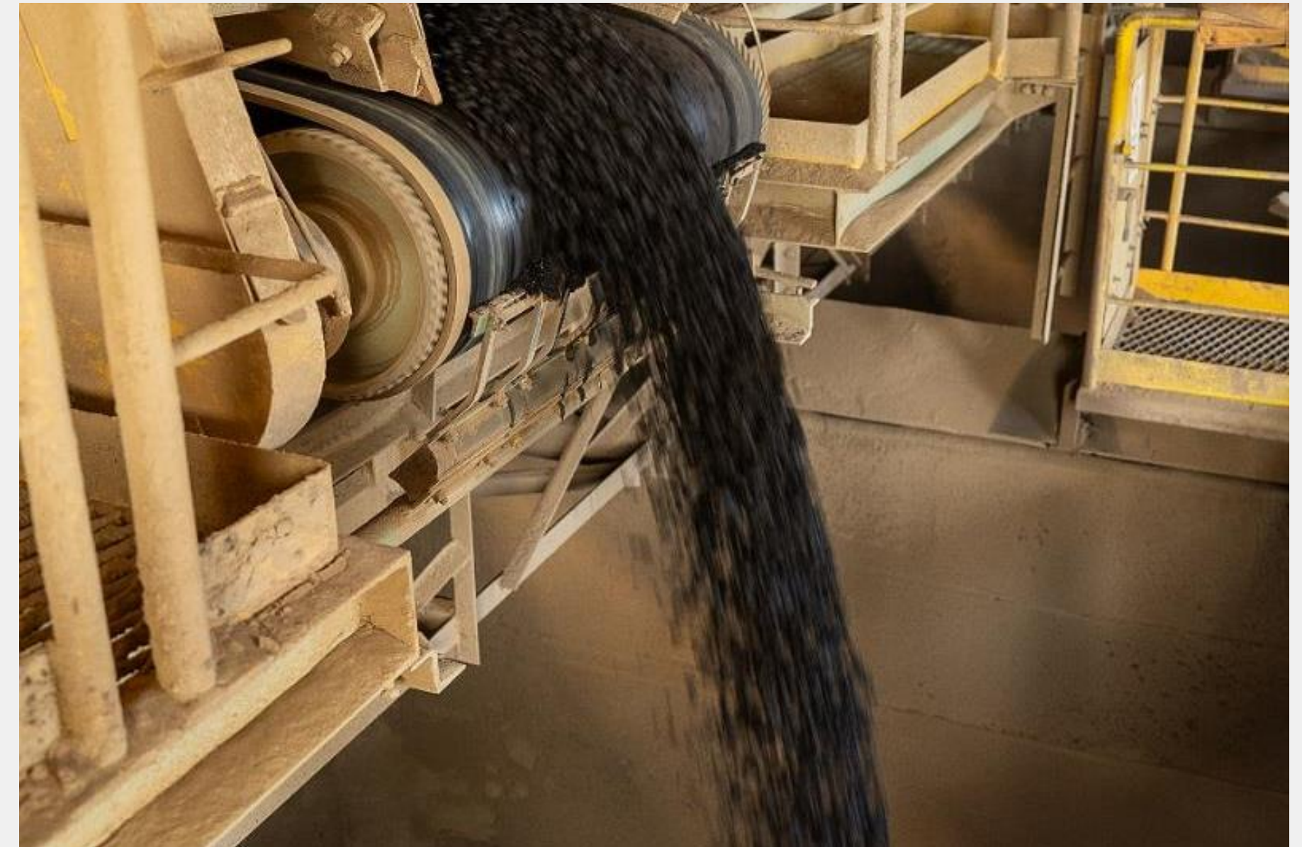
Calcine exits the Rotary Kiln #6 during industrial scale calcining campaign
