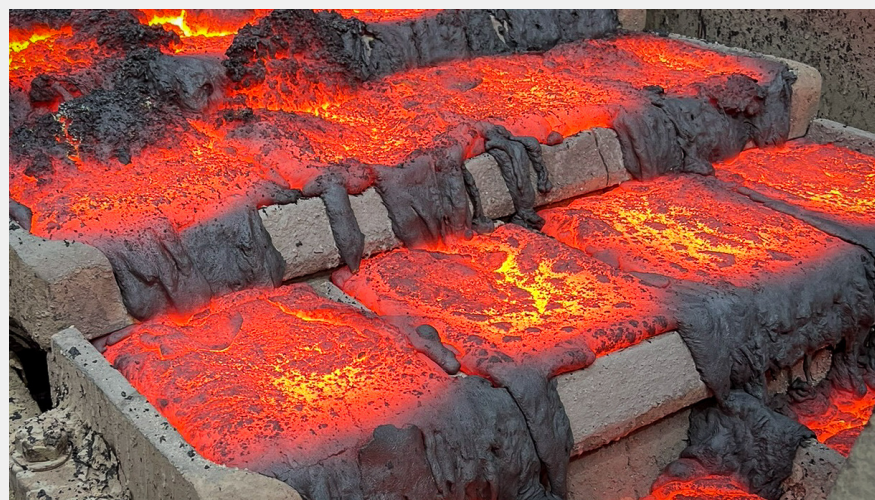
High-grade nickel-cobalt-copper alloy poured into ladles after smelting
