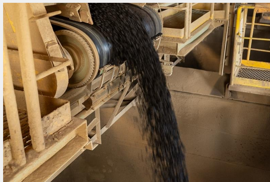
Calcine exits the Rotary Kiln #6 during industrial scale calcining campaign
