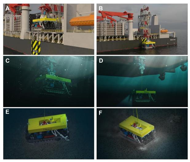
When lowering the PCV through the splash zone, the vessel heading will be adjusted such that the LARS is on the lee side, and wave shielding is provided to the LARS. This is done to reduce the splash zone loads, as illustrated in Figure 3-20. When the PCV has passed through the splash zone, the heading will be adjusted to bow incoming waves again.
