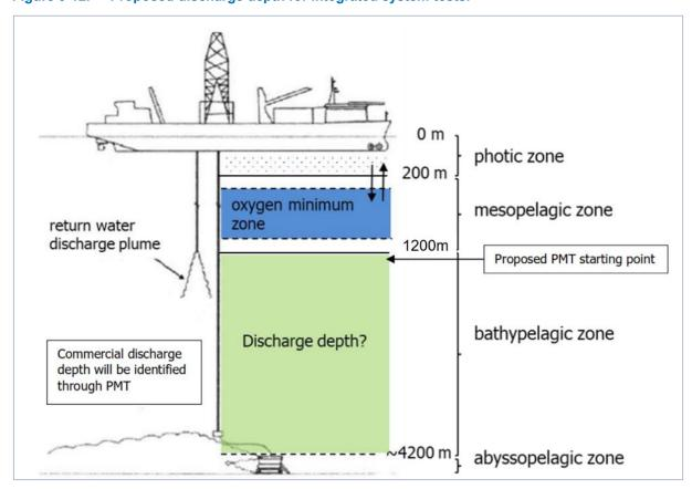
Figure 3-12. Proposed discharge depth for integrated system tests.
