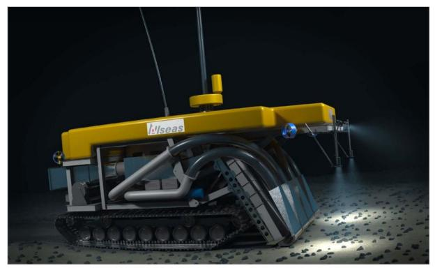
The PCV has been designed to collect nodules from the seafloor and transfer them to the base of the riser system which transports them to the SSV. The PCV design has been structured around five core functions that the vehicle must be capable of executing in order to collect and transfer nodules:
