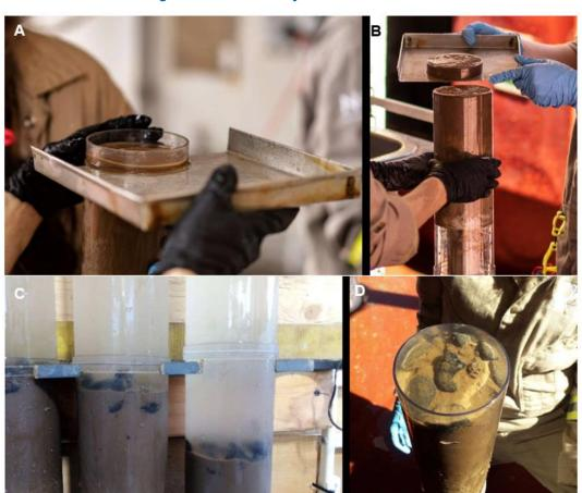
Figure 6-10. Sediment slicing for meiofauna analysis.
